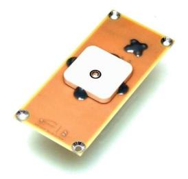
Fig. 1 Micro GPS-L1 Patch Antenna - Flight Model.
