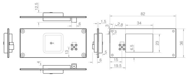
Fig. 2 microPATCH-L1 Dimensions drawing, standard MCX right-angle configuration depicted.
