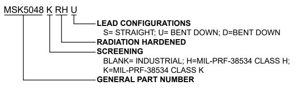
The above example is a Class K switching regulator with leads bent up. NOTE: See DLA SMD 5962R11232 for DLA part number options.
