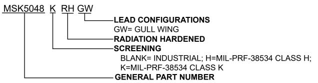
The above example is a Class K switching regulator with gull wing leads.
