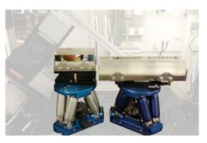
Two BORA hexapods position Kirkpatrick-Baez (KB) mirrors with high stability and resolution to improve the beam quality on a synchrotron beamline.
