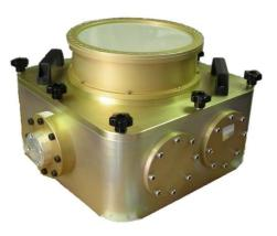
The re-configurable access ports include a large 200 mm vacuum window on the top plate made of Mylar and PTFE, ideal for IR direct signal reception (e.g. a satellite feed). The window and its extension tube can be removed and replaced by a metal blank plate with sealing ring.
