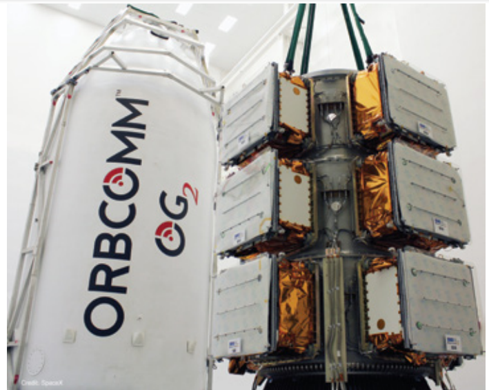
The final operational OG2 launch in December 2015 was the first time three Evolved Expendable Launch Vehicle (EELV) Secondary Payload Adapters (ESPA) were stacked for a constellation deployment.
