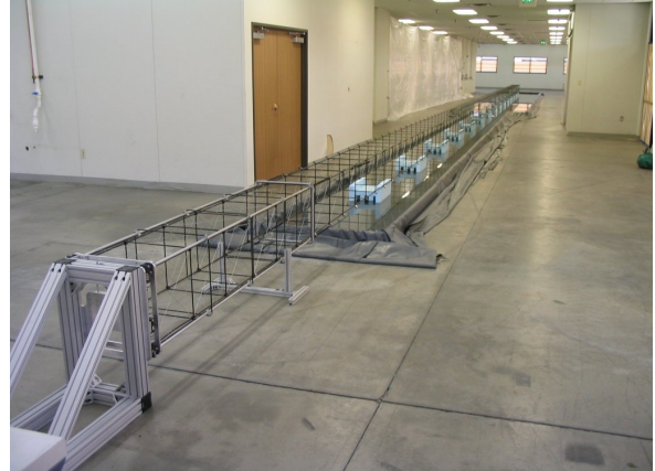
Jackscrew Deployed Boom Under Test
