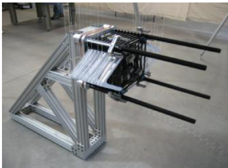
10-Bay Jackscrew Deployed Boom (stowed)
