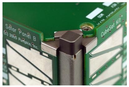
The image above shows one corner of a CubeSat Kit with its Solar Panel Clip installed, with panels (not included) made from 0.062" (1.5mm) PCB material. Each clip fits between a Cover Plate (shown) or Base Plate and the associated foot, and is held in place via the foot screw (not visible).
