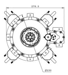
Redundant two phase bipolar stepper
