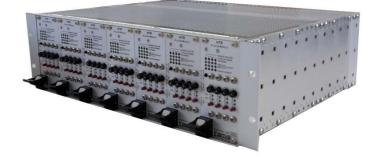
The POWER Box is in charge to provide power supply lines towards the UUT simulating the power distribution unit. The box has been designed to host, in any mixed configuration, two kind of plug in modules:
