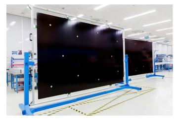
Airborne has delivered over 300 state-of-the-art solar-array substrates to several paramount European satellites. We develop and qualify affordable substrate panels for mega-constellations. Offering a disruption in price and production volume of panels.
