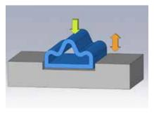
6. Profile for significant targeted displacement and minimal compression force
