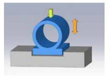
5. Profile for medium targeted displacement and weak compression force
