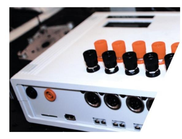
EGSE specifically designed to **support REACT operations during on-ground activities** such as validation/acceptance test at device and system level.
