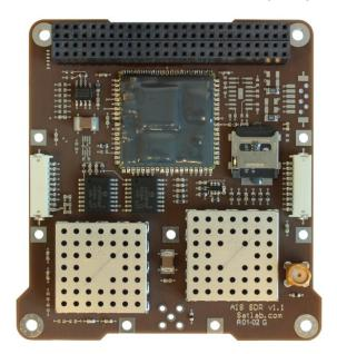
Figure 10: Top view of the QubeAIS with SMA straight in the RF1 connector placement
