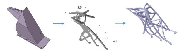
Structural design capabilities cover a broad area including material, coating and standard part selection, 3D design of metallic and CFRP parts, composite design, 3D tolerance analysis, structural budgets, system layout and equipment accommodation. Innovative design and manufacturing solutions like the design for additive manufacturing are also in the scope of the team.
