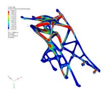
Robust design development and verification with the helpof finite element analysis is performed for the wide range of analysis types like topology optimization, static, dynamic, thermo-elastic, and vibro-acoustics. Structural and thermal tests predictions, test planning and mathematical model correlations are also part of the hands-on experience.
