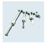
Single axis adapters for dovetail, fir tree, and round hole blade roots. Space Electronics "Gravity Wedge" Blade Adapters are more repeatable and easier to use than
