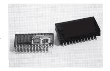
Low Power — CMOS proprietary monolithic devices in a unique circuit configuration yield the lowest power of any 16-Bit converter available.
