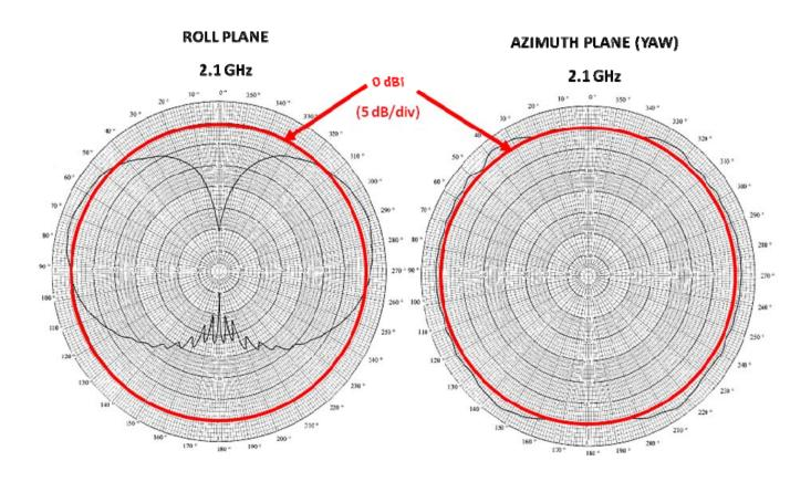
Note: Measured on a smooth cylindrical groundplane. Fins and other protrusions on the vehicle will perturb the radiation pattern. The extent of any perturbations cannot be fully determined until radiation patterns are either calculated or measured on a model of the vehicle. Haigh-Farr offers engineering services, which include the calculation of radiation patterns on a specific vehicle.
