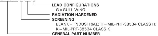
The above example is a Class K regulator with gull wing formed leads. NOTE: See DSCC SMD 5962F09208 for DSCC part number options.
