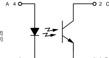
ANODE ELECTRICALLY CONNECTED TO CASE.
