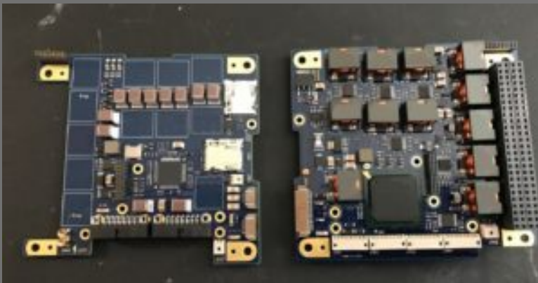
ExoTerra's Power Distribution Card can process 1 kw on a PC 104 board
