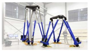
FMC Technologies uses two SIROCCO XL hexapods to test a ¼ scale LNG loading arm. These hexapods simulate the swell motion to qualify the loading arm that will connect a gas carrier to an offshore gas production factory. One hexapod simulates the gas carrier, the other the offshore factory.
