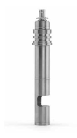
signal. When the gap between the transmitter and receiver is filled by a liquid medium, the vibration generated in the transmitter is transmitted to the receiver. The change in the signal level enables the electronic control unit (separate unit) to sense the presence or absence of the liquid. The amplitude of the output signal depends upon the type of the medium present across the sensing gap.
