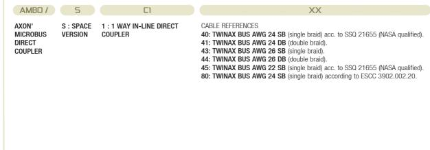
NOTE: CABLE LENGTH AND CABLE COLOUR TO BE DEFINED WHEN ORDERING (possibility to differentiate bus and stub cable with a striped colour tape under the transparent jacket or the extrusion of a colour jacket).
