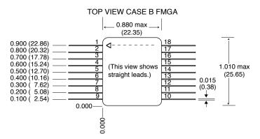
The triangle (ESD) marking on the cover indicates pin one. Cover marking is oriented with pin one at the upper right corner. The straight lead configuration does not require a "case designator" in the model number. ex. FMGA-461
