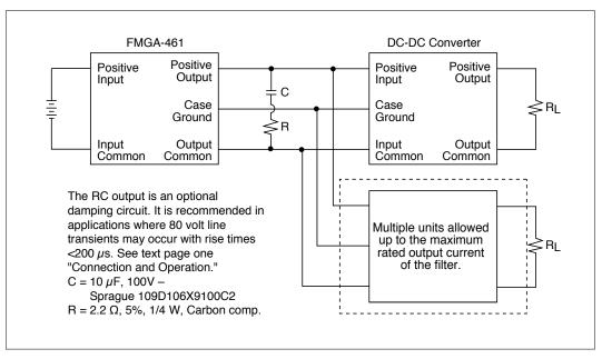
FIGURE 3: FMGA DAMPING CIRCUIT
