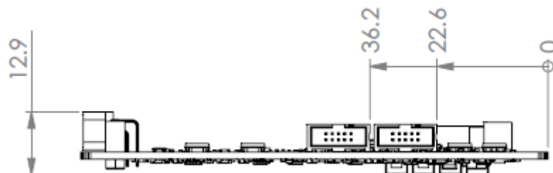
Figure 7: Mechanical Drawing of NANOif – Side view
