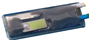
Figure 10: Photodiode Soldered onto Small PCB
